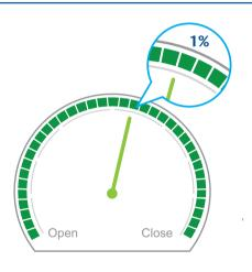
≤1% guaranteed accuracy when the valve needs to be precisely positioned. 4-20mA analog input and output to provide both precise control and instantaneous feedback. Precise Hall-Effect position encoder; provides consistent and accurate position feedback with no loss of calibration during power failures.
